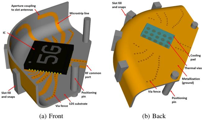
Fig. 2: LDS-MID with beamforming IC and cooling pad
