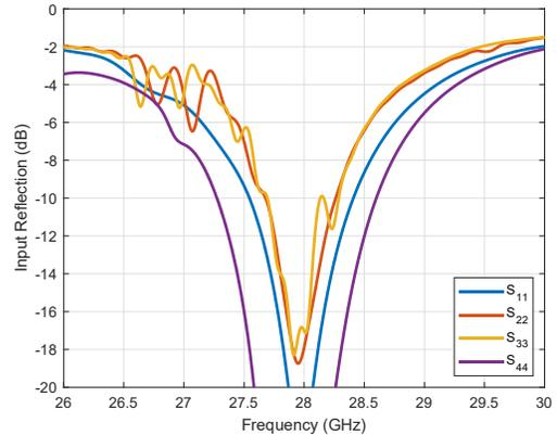
Fig. 3: Input reflection coefficients at microstrip feed lines inside metal smartphone chassis
