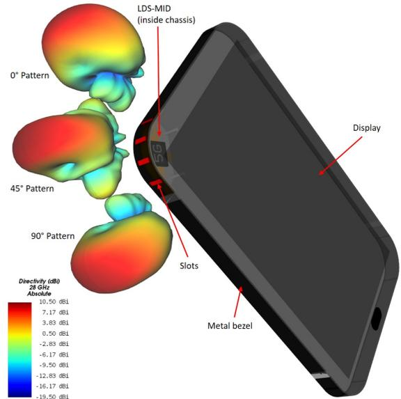
Fig. 1: Smartphone chassis with four-slot-array realized in the upper-left corner of the metal bezel and exemplary radiation patterns achieved by different settings of the beamformer
