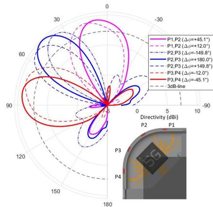
Fig. 4: Beam steering pattern with labeling of active ports (P1,P2,P3,P4) and phase difference  $\Delta\phi$  between ports
