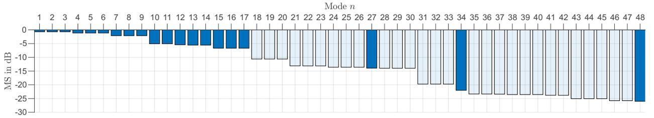
Fig. 4. Modal significance of the first 48 modes on the cube. Modes not used for the DoA estimation are displayed as transparent bars.
