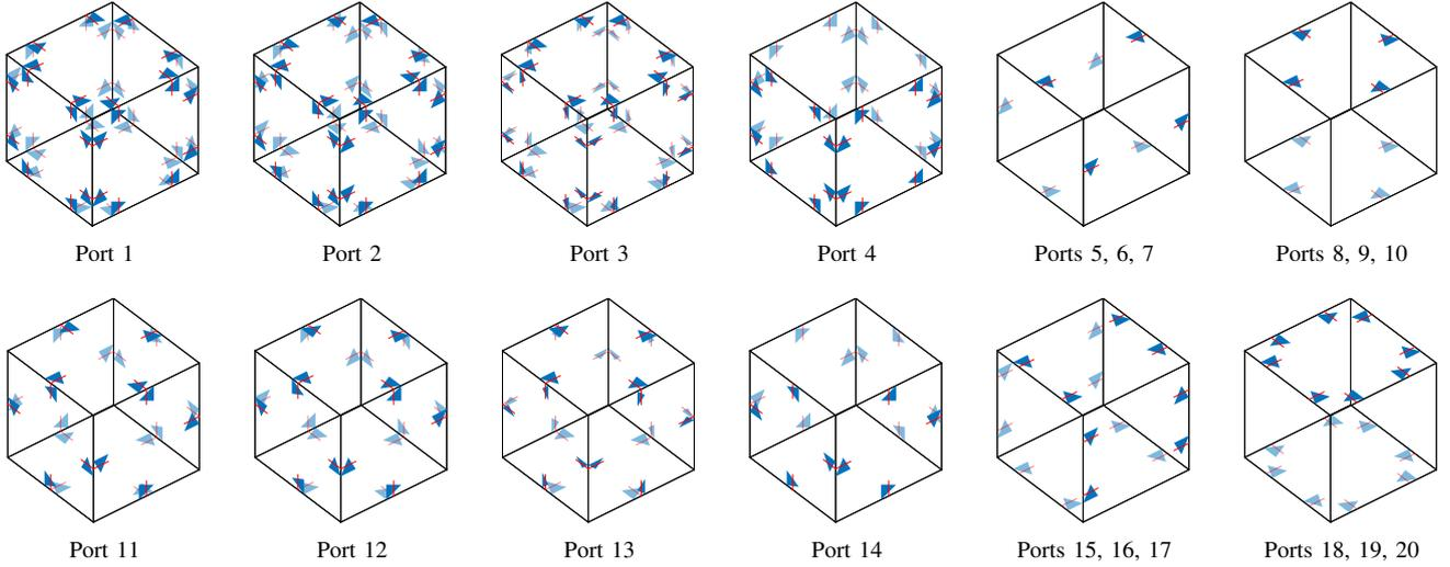
Fig. 1. Feed setups for 20 uncorrelated ports on a cube. Where multiple port numbers are given, the last two can be obtained from the displayed first one by rotating around the main axis. For ports 3 and 13, some feeding points only have half the amplitude of the other ports, which is marked with shorter arrows.
