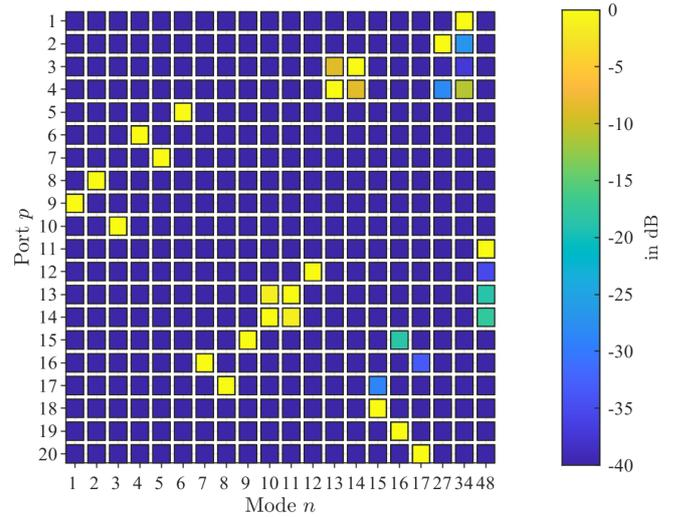
Fig. 5. Magnitude of the entries in the port-mode matrix  $I_{\text{ports},CM,p,n}$  of the selected setup, normalized to the maximum value of each port.
