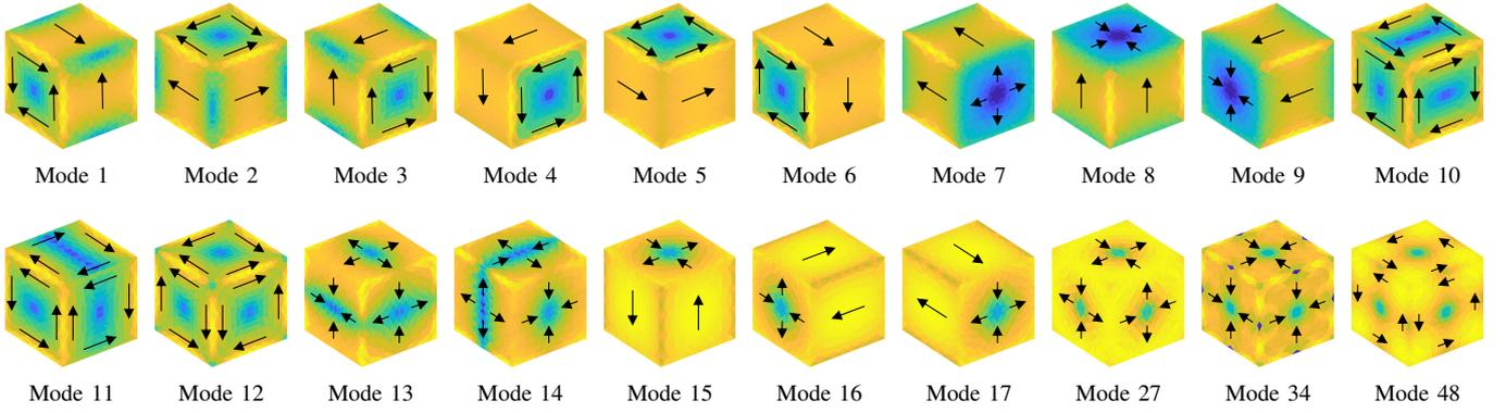
Fig. 3. Selection of characteristic mode current densities supported by the cube. For scale refer to the colorbar in Fig. 5
