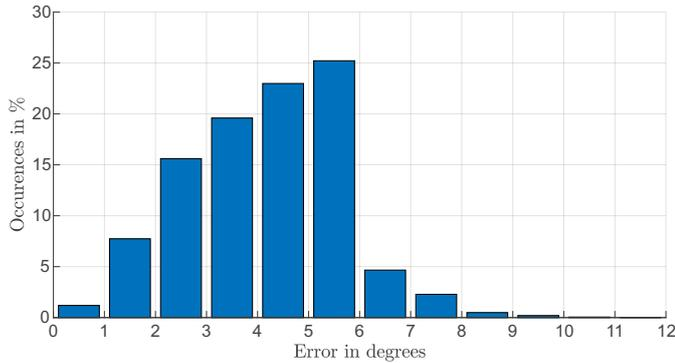
Fig. 6. Distribution of errors of the estimated DoA for the proposed example setup, obtained by using randomly distributed DoAs for testing. Based on the reference data, the accuracy is roughly 7 degrees.
