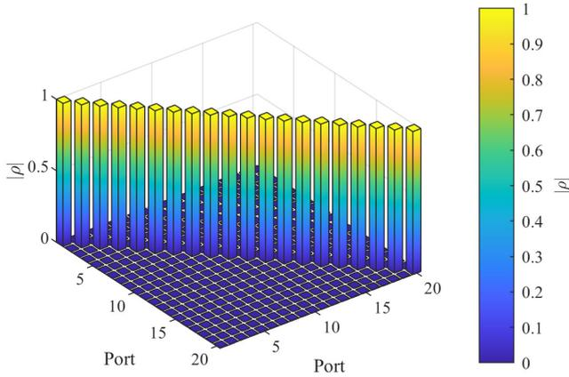
Fig. 2. Envelope correlation coefficient of ports.
