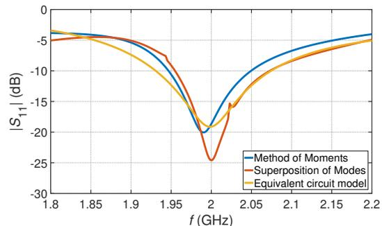
Fig. 5.  $S_{11}$  of a smartphone antenna compared to the superposition of dominant modes and an equivalent circuit model.
