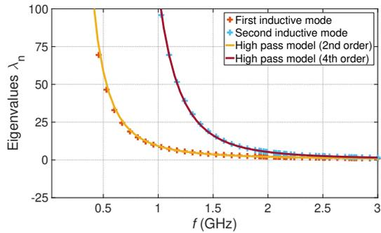
Fig. 3. Eigenvalues for inductive modes of a thin PEC plate compared to circuit models based on inductive high passes.
