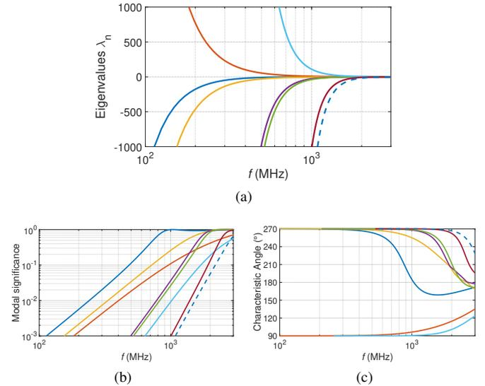
Fig. 2. (a) Eigenvalues, (b) modal significance and (c) characteristic angle of a 130x70 mm<sup>2</sup> thin PEC plate.
