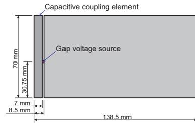
Fig. 4. Model of a generic smartphone chassis with a capacitive coupling element and a gap voltage source.
