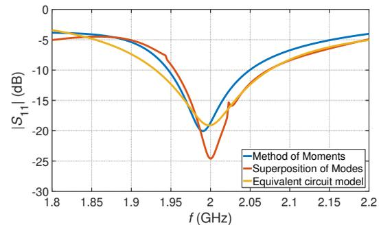
Fig. 5.  $S_{11}$  of a smartphone antenna compared to the superposition of dominant modes and an equivalent circuit model.
