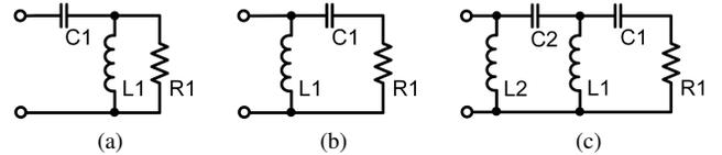
Fig. 1. High pass equivalent circuit models. (a) Second order capacitive high pass (HP2-CAP). (b) Second order inductive high pass (HP2-IND). (c) Fourth order inductive high pass (HP4-IND).
