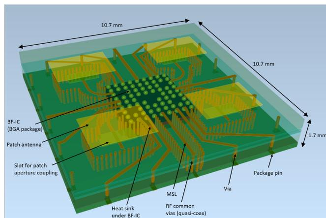
Fig. 1. Integrated multilayer structure for a BF-IC with four patch antennas. Inter-element distance is half a free-space wavelength
