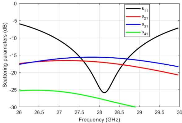
Fig. 3. Simulated scattering parameters (reference impedance 50Ω) for input at BGA contact point of antenna 1. Antennas 2 and 3 are neighbored to antenna 1.
