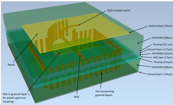
Fig. 2. Aperture coupled patch antenna in multilayer structure.
