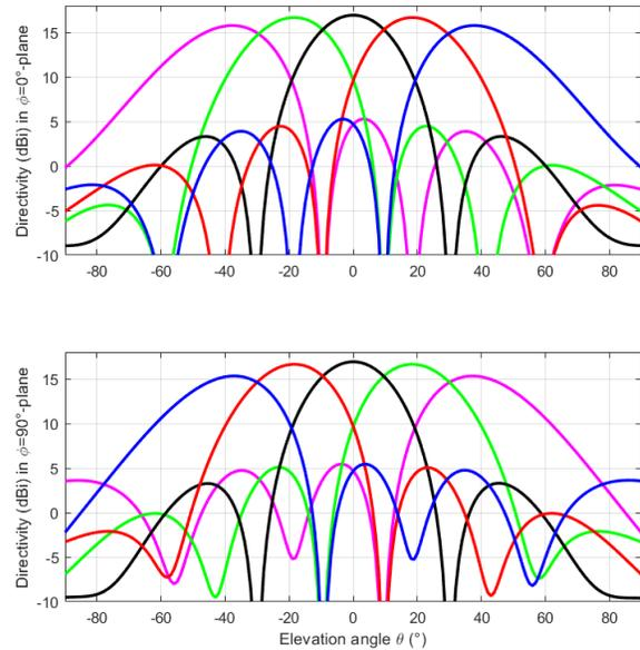
Fig. 6. Directivity of a four tiles with beam steering over elevation angle in  $\phi = 0^\circ$ -plane and in  $\phi = 90^\circ$ -plane (azimuth angle).
