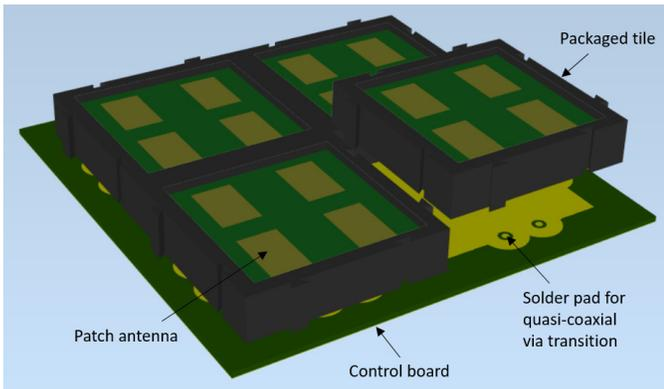
Fig. 5. Four packaged 2x2-antenna modules (tiles) placed on control board to get a 4x4 antenna array.
