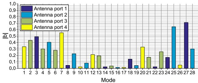
Fig. 6. Normalized modal weighting coefficients of rectangular PEC plate excited according to Table IV at 7.25 GHz.
