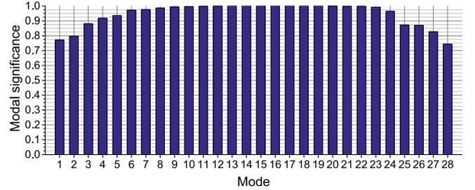
Fig. 2. Modal significances of rectangular PEC plate at 7.25 GHz.
