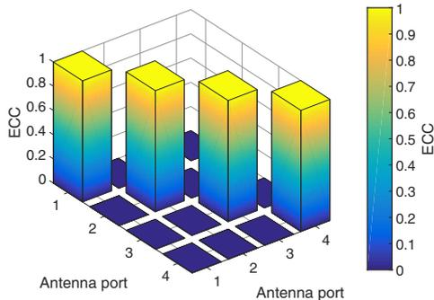
Fig. 7. Envelope correlation coefficients (ECC) of antenna ports according to Table IV at 7.25 GHz.
