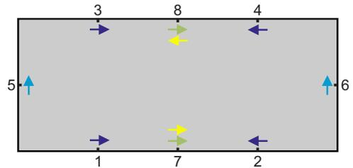
Fig. 5. Voltage source locations and feed directions on rectangular PEC plate.
