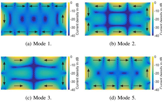
Fig. 3. Normalized surface current densities of four significant characteristic modes of rectangular PEC plate at 7.25 GHz.
