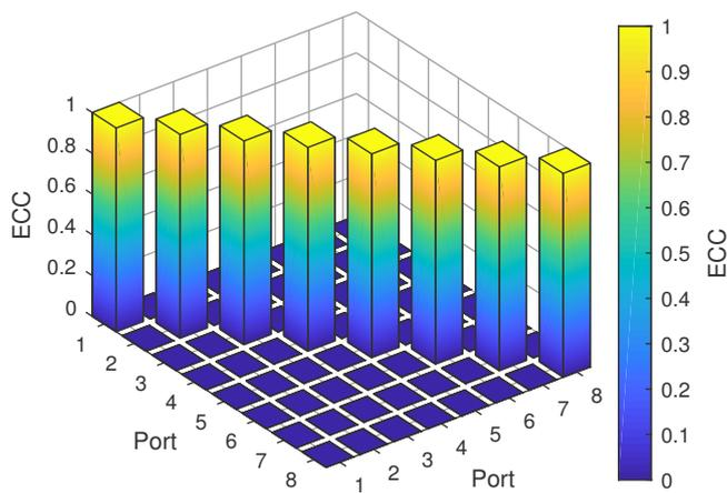
Fig. 7. Envelope correlation coefficients (ECC) of hexagonal PEC plate excited according to Fig. 5.
