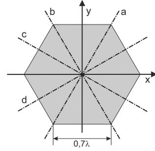
Fig. 1. Hexagonal plate and coordinate system.
