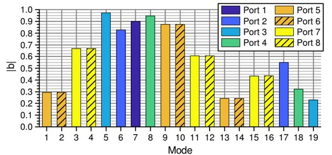
Fig. 6. Absolute values of normalized modal weighting coefficients  $b$  of hexagonal PEC plate excited according to Fig. 5.
