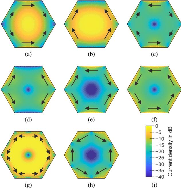
Fig. 2. Normalized surface current densities of significant characteristic modes of hexagonal PEC plate with principal current directions at the edges denoted by arrows. (a)-(h) Modes 1 to 8. (i) Colorbar.
