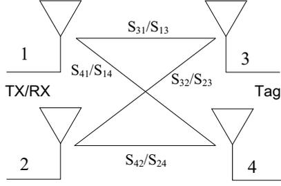
Figure 2. Scheme of the  $2 \times 2 \times 2$  MIMO RFID system
