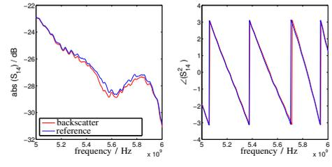
Figure 9. Backscatter and reference measurement results for  $S_{14}$
