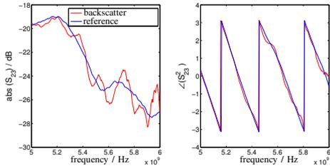
Figure 8. Backscatter and reference measurement results for  $S_{23}$
