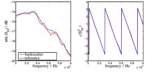
Figure 10. Backscatter and reference measurement results for  $S_{24}$
