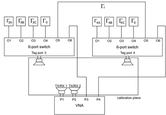
Figure 5. Measurement setup:  $2 \times 2 \times 2$  backscatter system
