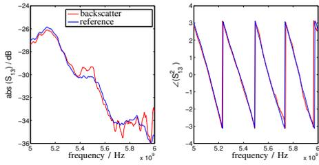
Figure 7. Backscatter and reference measurement results for  $S_{13}$
