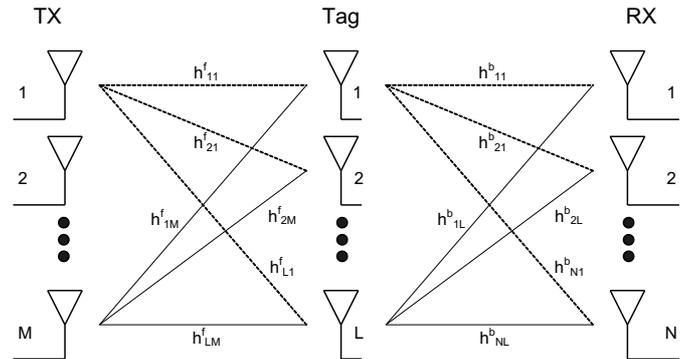
Figure 1.  $M \times L \times N$  MIMO RFID system
