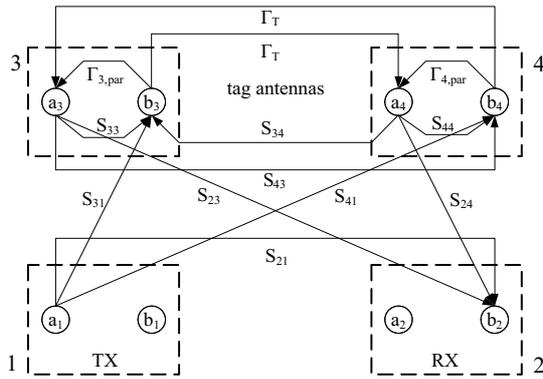
Figure 4. Signal-flow graph of the  $2 \times 2 \times 2$  system for tag termination with  $\Gamma_T$  for one pair of TX/RX-antenna ports at 1,2
