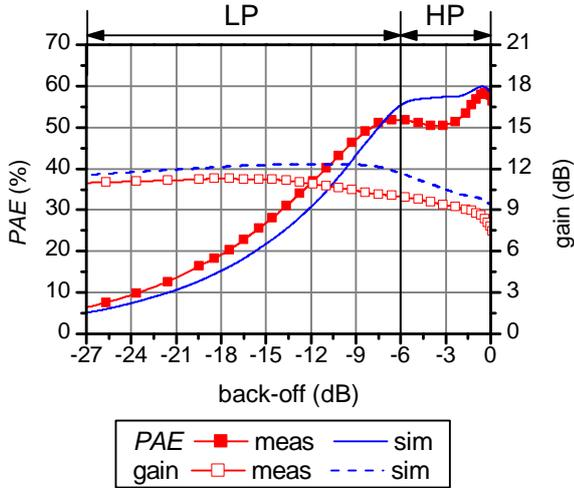
Fig. 5. Measured and simulated  $PAE$  and gain versus back-off for the offset line  $TL_{off,3-}$ .
