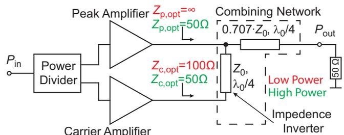
Fig. 1. Block diagram of a Doherty power amplifier.
