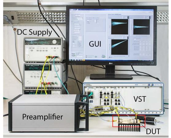
Fig. 6. Measured setup for the DPD based on a NI vector signal transceiver.
