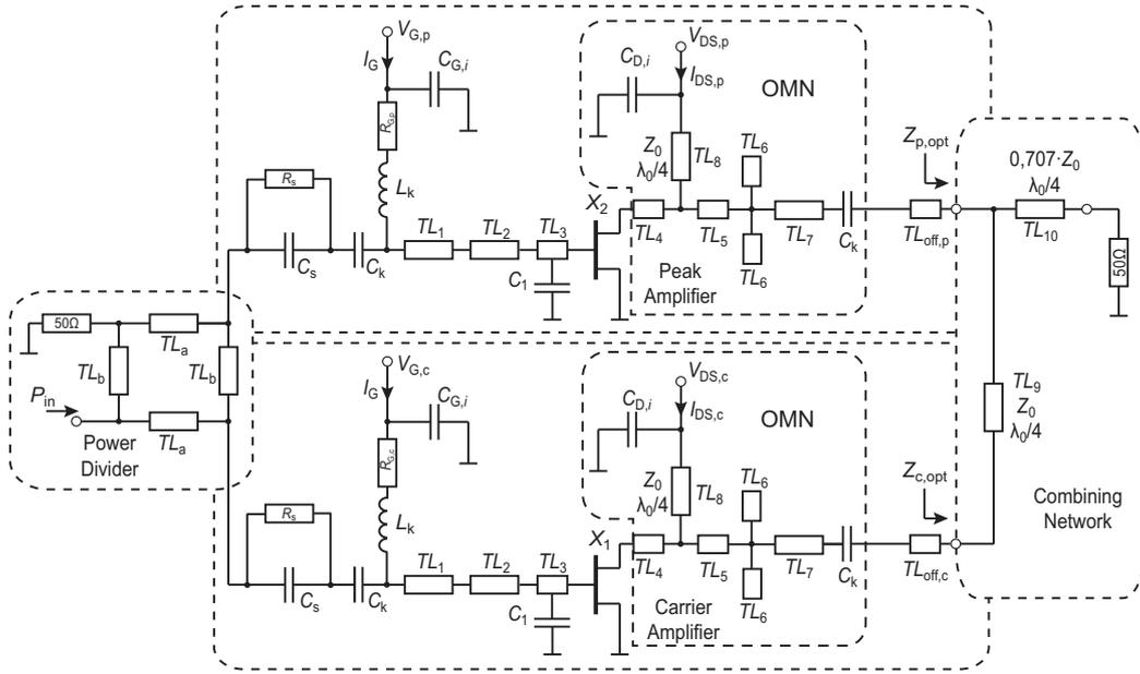
Fig. 2. Schematic of the developed Doherty amplifier.
