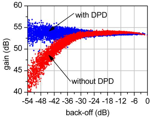
Fig. 7. Measured gain curve (AM-AM) without and with memoryless DPD.
