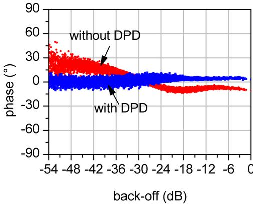
Fig. 8. Measured phase (AM-PM) without and with memoryless DPD.
