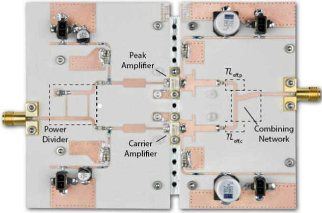
Fig. 4. Photo of the developed Doherty power amplifier.
