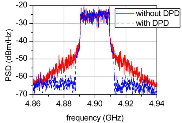
Fig. 10. Measured power spectral density of a 20 MHz 64-QAM-OFDM signal without and with memoryless DPD.
