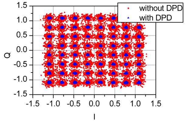
Fig. 9. Measured 64-QAM constellation without and with memoryless DPD.
