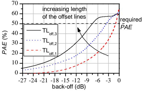
Fig. 3. Simulated *PAE* versus back-off for various offset lines lengths.
