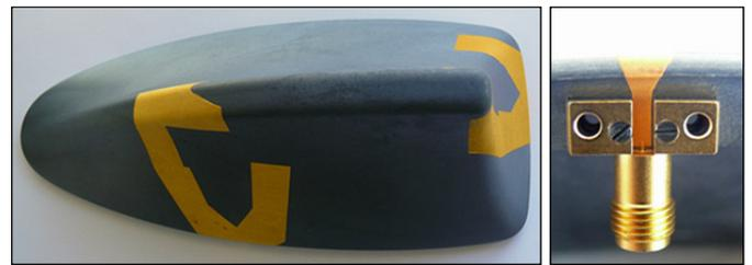
Fig. 12 Realized two-antenna system with feeding structure
