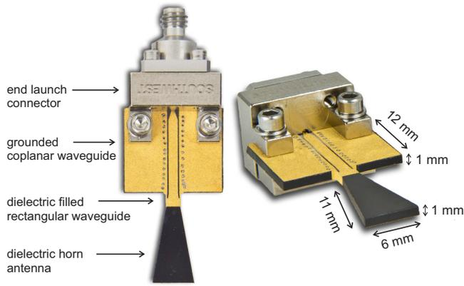
Fig. 3. LDS fabricated test antenna
