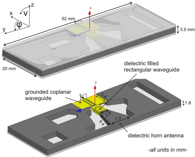
Fig. 6. Simulation model of integrated smart device antenna
