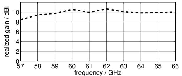
Fig. 9. Simulated realized gain over frequency
