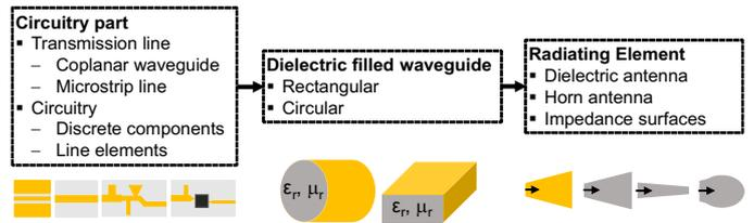
Fig. 2. Possible waveguide fed antenna configurations
