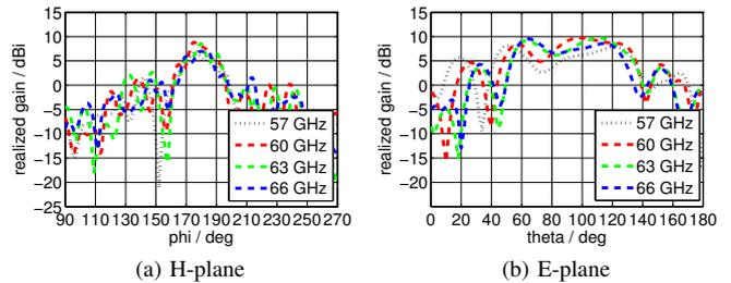
Fig. 8. Simulated radiation characteristics of the integrated smart device antenna
