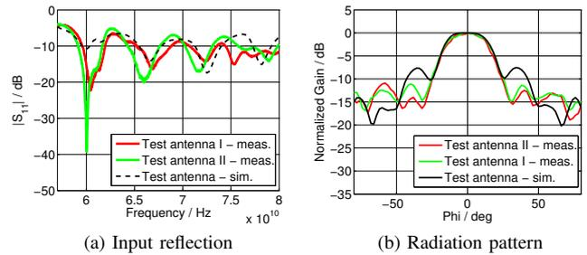
Fig. 4. Measured and simulated characteristics of the test antenna
