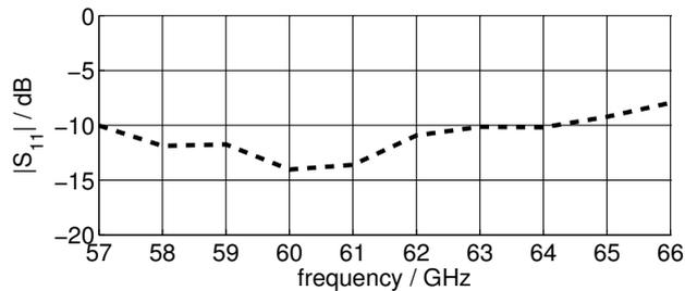
Fig. 7. Simulated input reflection of integrated waveguide fed antenna
