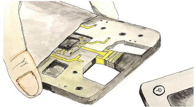
Fig. 5. Schematic sketch of future smart device containing 3D integrated waveguide fed antenna
