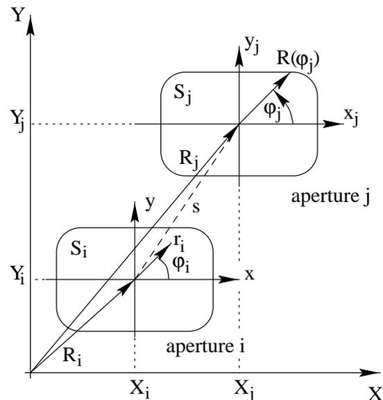
Fig. 1: GEOMETRY OF CYLINDRICAL WAVEGUIDES OPENING INTO A GROUNDPLANE
