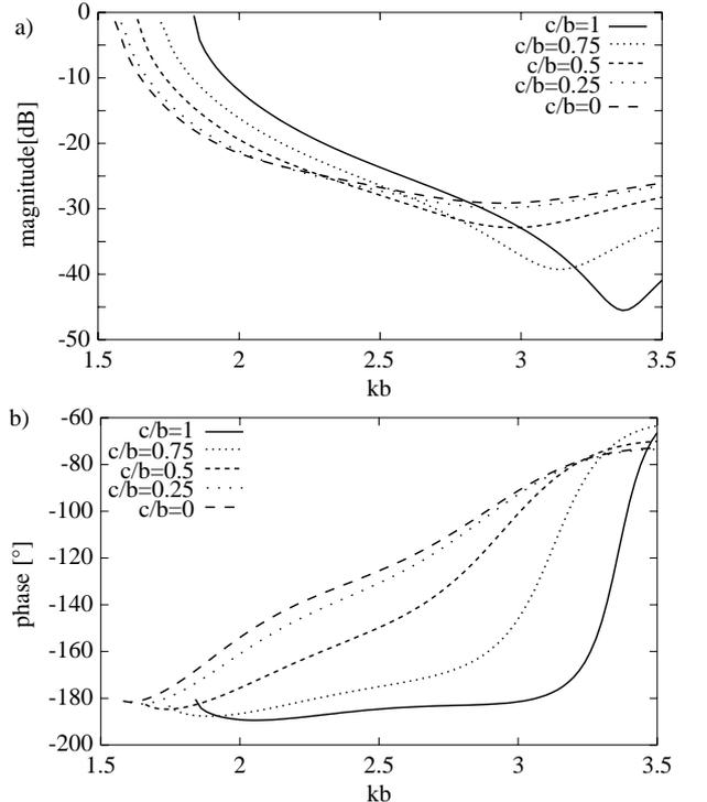
Fig. 4: REFLECTION COEFFICIENT OF TE<sub>1</sub> MODE AGAINST NORMALIZED FREQUENCY
