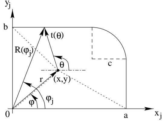
Fig. 3: COORDINATE-TRANSFORM FOR EVALUATING THE SINGULARITY
