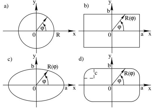
Fig. 2: GEOMETRY OF THE CROSS-SECTION OF DIFFERENT CYLINDRICAL WAVEGUIDES; a) CIRCULAR b) RECTANGULAR c) ELLIPTICAL d) RECTANGULAR WITH ROUNDED CORNERS
