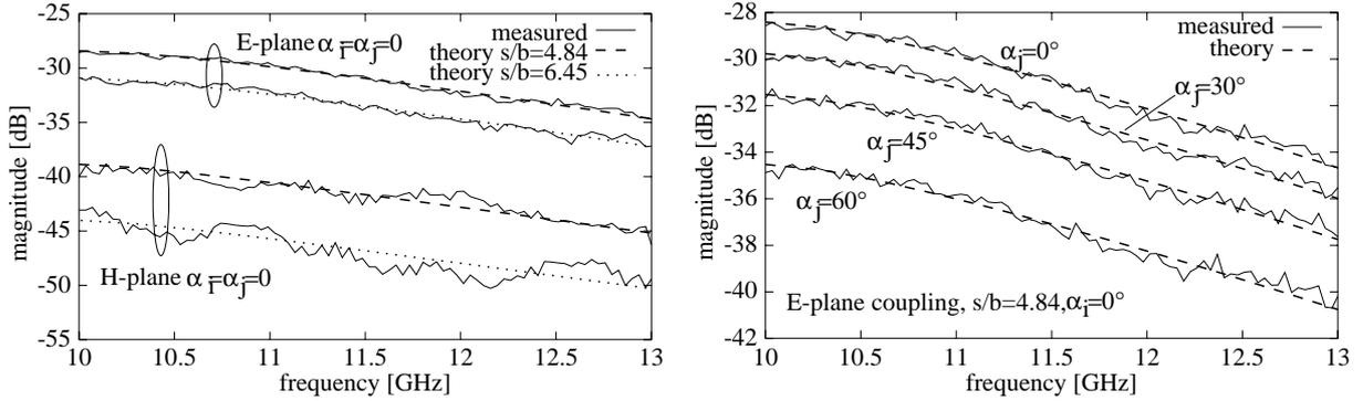
Figure 4: Coupling coefficient for waveguides with  $a=b=c$  ( $\equiv$  circular cross-section)
