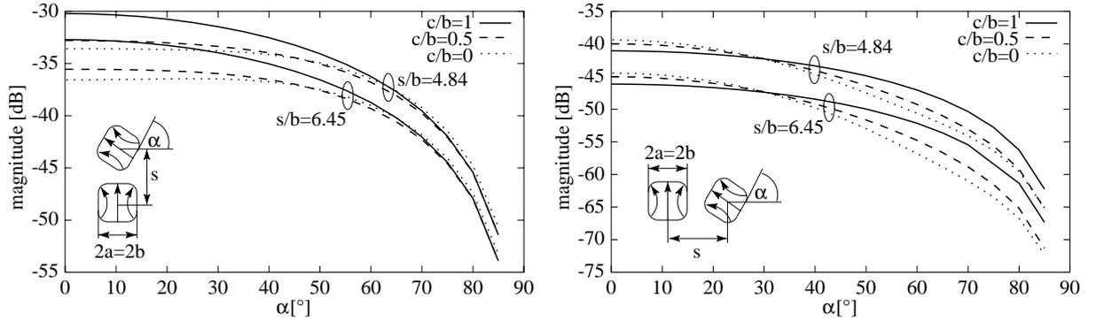
Figure 3: E-Plane and H-plane coupling for identical waveguides against rotation angle  $\alpha$  at  $kb = 2.2$
