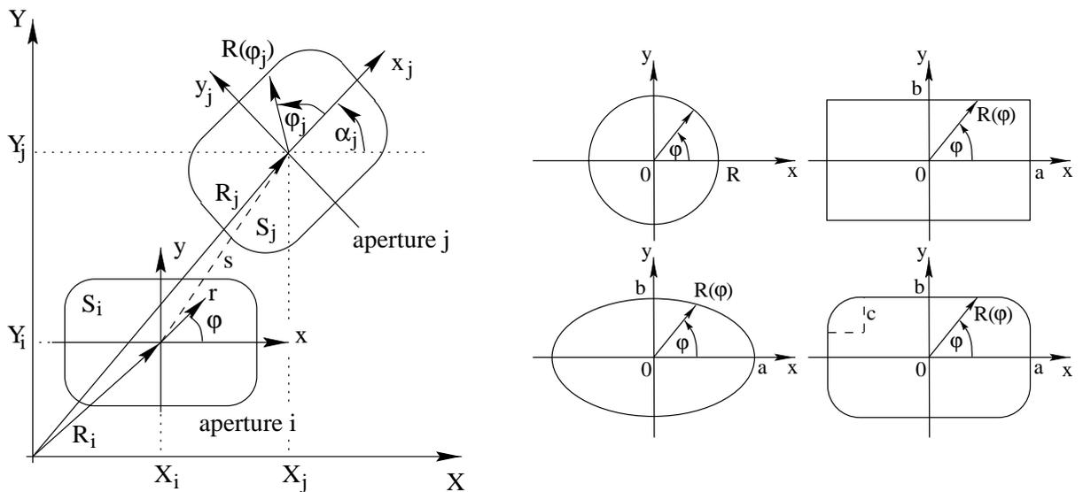
Figure 1: Geometry of cylindrical waveguides opening into a ground plane
