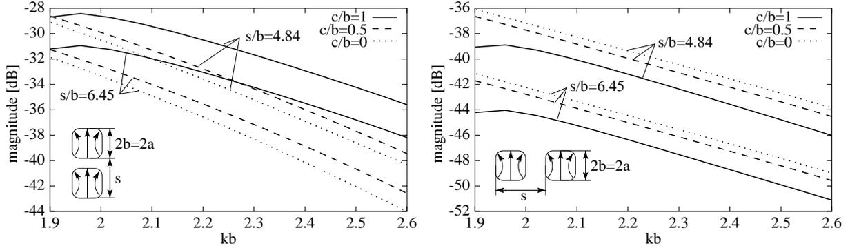
Figure 2: E-Plane and H-plane coupling for identical waveguides against normalized frequency
